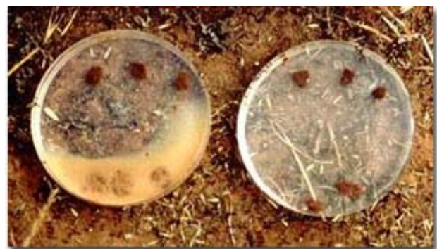
Figure 1. Soil aggregates in distilled water (left) and distilled water plus gypsum solution (right)
